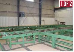
(2) 54" x 120' Hydraulic Power Roller Transfer Conveyors
